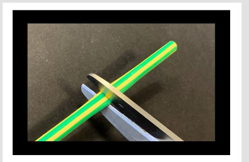
Start by cutting the liner to the correct length for the surface to be protected, taking into account the longitudinal shrinkage of around 5%.
