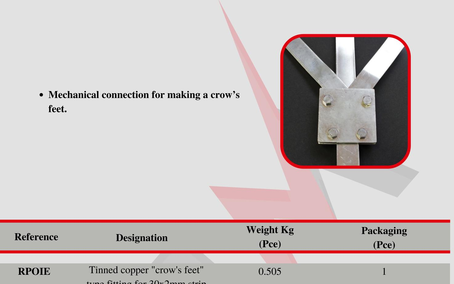
type fitting for 30x2mm strip up to 30x3.5mm. Tightening by 4 M8x25 stainless steel A2 bolts.
